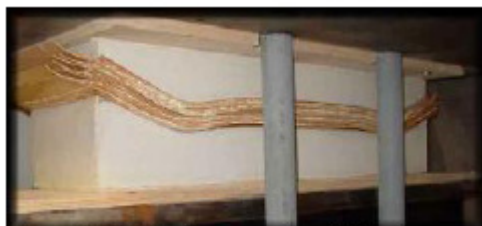
Figure 1.2.3: Maple veneers in a hydraulic press
