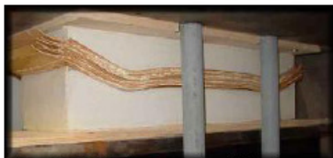
Figure 1.2.3: Maple veneers in a hydraulic press
