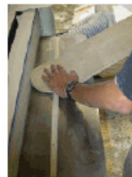
Figure 1.2.4: Shaping a deck
